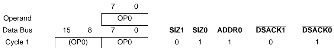
Figure 5-10 Byte Operand to 16-Bit Port, Odd (ADDR0 = 1)
